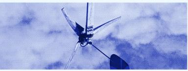
A wooden rotor and tower greatly increase the net energy output over the lifetime of a small wind turbine.
